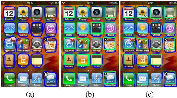
Figure 3. (a) Contours detects by our system. (b) Candidate bounding-boxes matched to the contours. (c) The final detected boxes
