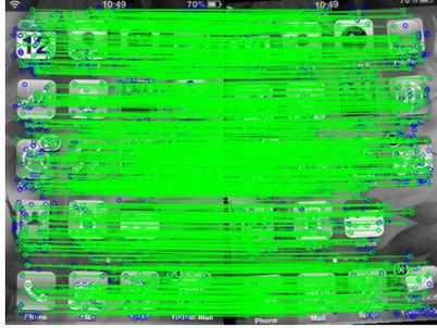
Figure 2. To align a pair of frames we fit a Homography using RANSAC and warp one of the frames.
